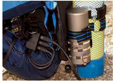
The control unit is strapped to the waist and the battery-pack to the tank
